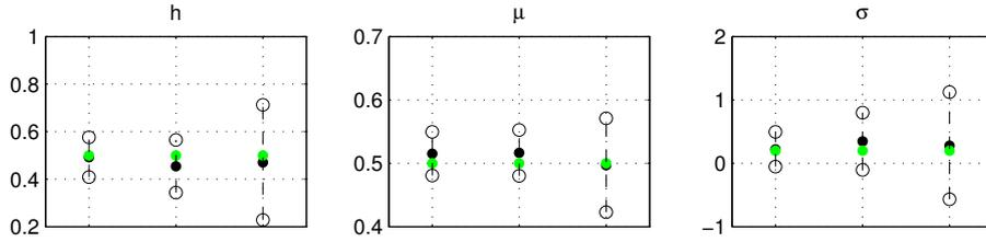
Figure 8: 99% CIs for the parameters  $h, \mu$ , and  $\sigma$ . In each plot from left to right, the sensors ( $m = 20$ ) are placed with uniform spacing on  $[0.1, 0.9]$ ,  $[0.1, 0.3] \cup [0.7, 0.9]$ , and  $[0.3, 0.7]$ . The true (estimated) parameter values are indicated with green (black) dots. The initial guess for the parameter estimates is equal to the true parameters.
