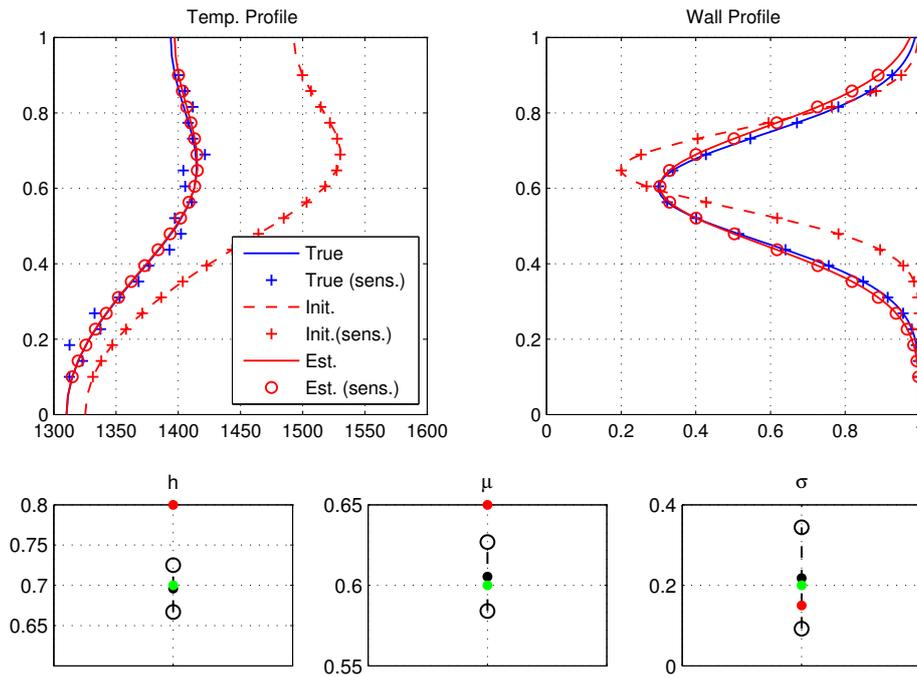
Figure 7: Top: The exterior temperature profiles (left) and corresponding wall profiles for the true parameters, the initial guess and the final estimates of the parameters. Bottom: The 99% CIs on each parameter. The initial and final parameter estimates are marked by the red and black dots resp. while the true value is marked in green. The true values are well within the 99% CI.
