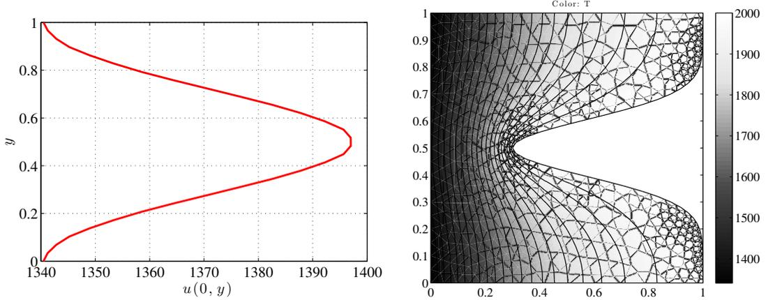
Figure 3: The exterior wall temperature profile (left) for the corresponding cross-sectional wall temperature profile (right) computed by solving the steady state heat equation (2.1) with boundary conditions (2.2). The interior wall shape profile  $w$  is given by (3.1) with  $(h, \mu, \sigma) = (0.7, 0.5, 0.15)$ .
