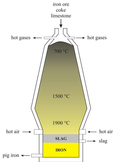
Figure 1: Blast furnace diagram
