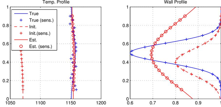
Figure 5: An example estimate of the inner wall profile for noisy data with wall parameters  $\underline{\mathbf{p}} = [0.4, 0.5, 0.15]^\top$ . Each sensor measurement is perturbed by normally distributed noise with mean zero and variance  $\zeta^2 = 3^2$ . The final parameter estimates were  $\hat{\underline{\mathbf{p}}} = [0.3064, 0.4850, 0.5113]^\top$ .
