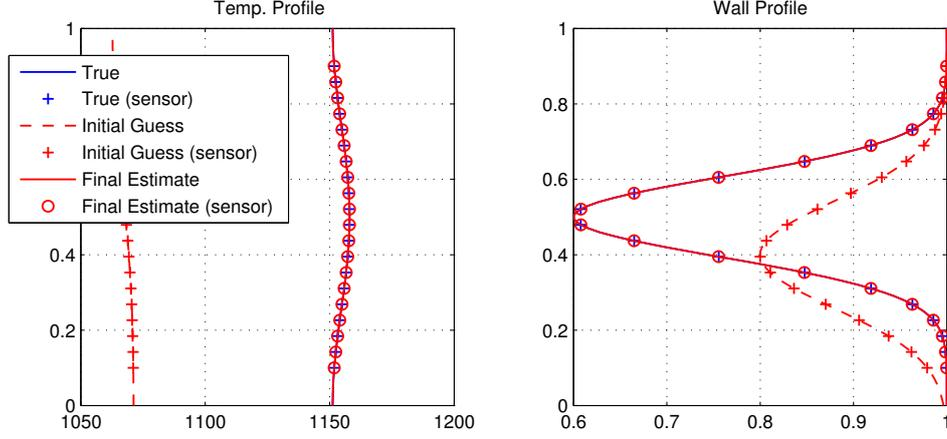
Figure 4: An example estimate of the inner wall profile for perfectly measured data with wall parameters  $\underline{\mathbf{p}} = [0.4, 0.5, 0.15]^\top$ . The relative error in each final parameter estimate is given by  $[0.1505, 0.0004, -0.8818]^\top \times 10^{-3}$ . The initial parameter “guesses” were  $\underline{\mathbf{p}}^{(0)} = [0.2, 0.4, 0.2]^\top$ . The positions of the 20 sensors are indicated with crosses and circles as the legend describes.
