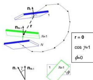
In testing for ring closure, an extra joining step  $N+1$  is added to the sequence. Configurations within chosen bounds of  $m=0$ ,  $\cos(\beta)=1$ , and  $\phi=0$  are used to approximate the  $J$  factor, which is equal to the value  $-\exp(\Delta G/kT)$ , and hence is well-suited to approximate the free energy of looping.
