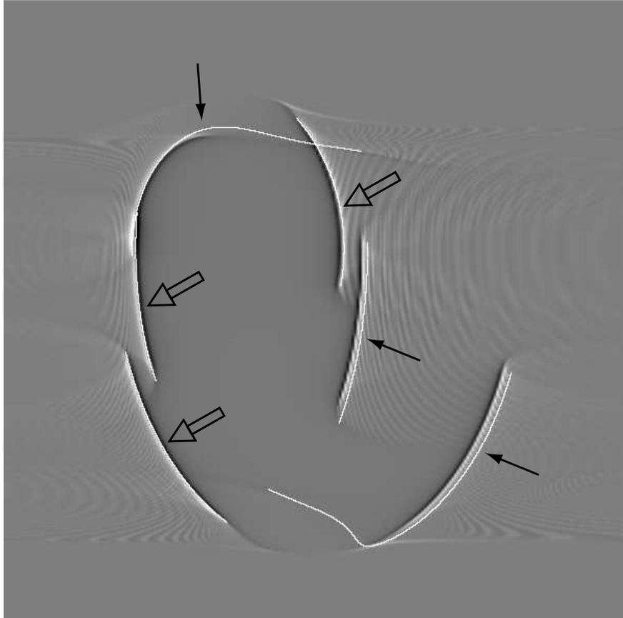
Illustration of the shift between the singularities of  $f$  and  $g$  in the dynamic case. The ellipsoid expands and contracts as well as moves left-right. The cross-section  $|x_1| \leq 75, x_2 = 0, -90 \leq x_3 \leq 60$  is shown.
