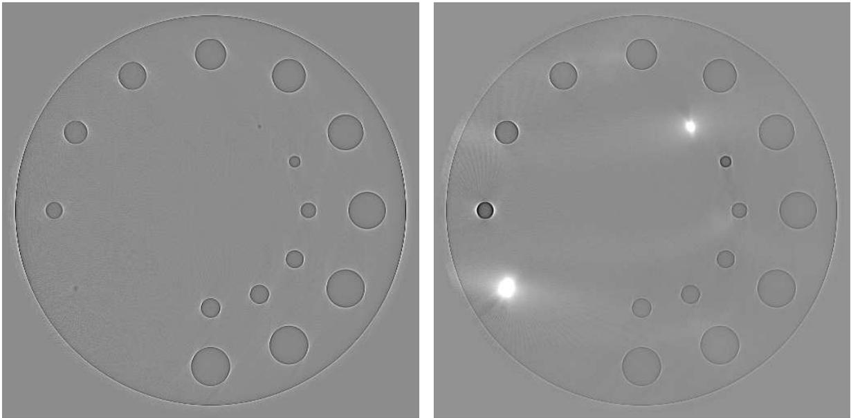
Reconstruction of the clock phantom. The cross-section  $|x_1| \leq 255.5, |x_2| \leq 255.5, x_3 = 0$  is shown. Left panel - new LT function  $g$ , right panel - old LT function  $g_\Lambda$ .
