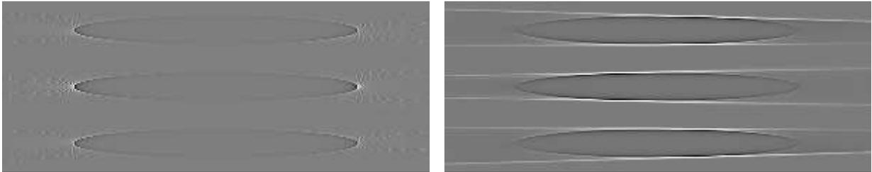
Reconstruction of the three-disk phantom. The cross-section  $|x_1| \leq 150, x_2 = 0, |x_3| \leq 60$  is shown. Left panel - new LT function  $g$ , right panel - old LT function  $g_\Lambda$ .
