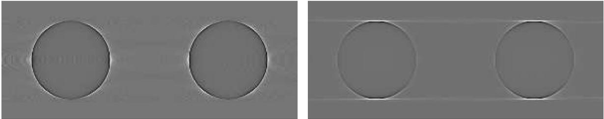
Reconstruction of the two-ball phantom. The cross-section  $|x_1| \leq 150, x_2 = 0, |x_3| \leq 60$  is shown. Left panel - new LT function  $g$ , right panel - old LT function  $g_\Lambda$ .
