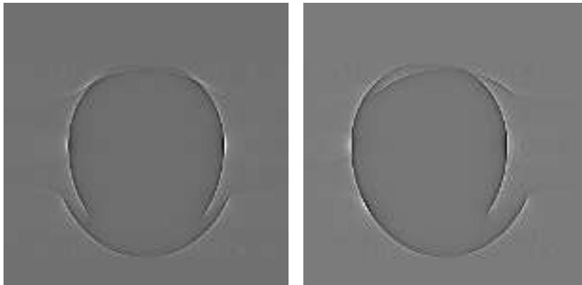
The ellipsoid either only expands and contracts (left panel) or expands and contracts as well as moves left-right (right panel). The cross-sections  $|x_1| \leq 75, x_2 = 0, |x_3| \leq 75$  are shown in both panels.
