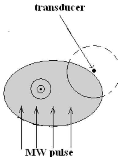
The integrals of the MW energy absorption function  $f(x)$  over circles centered at transducers' locations are measured.
