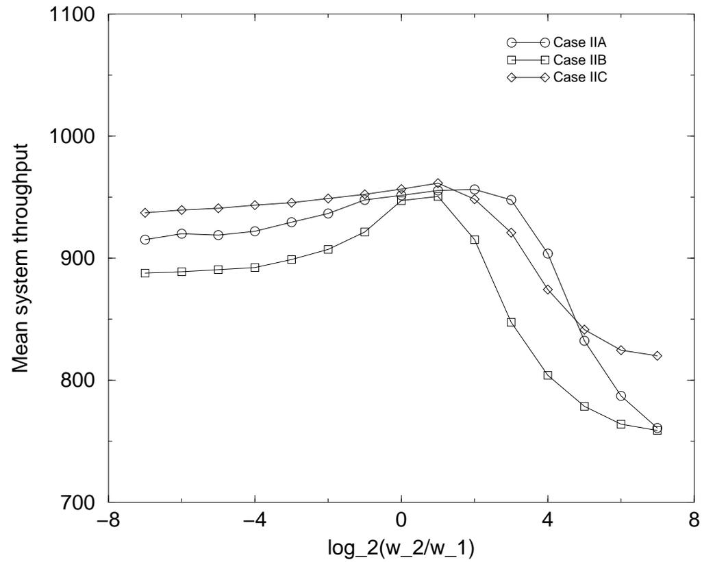
**Mean system throughput as function of  $\log_2(w_2/w_1)$  for Cases IIA-C**
