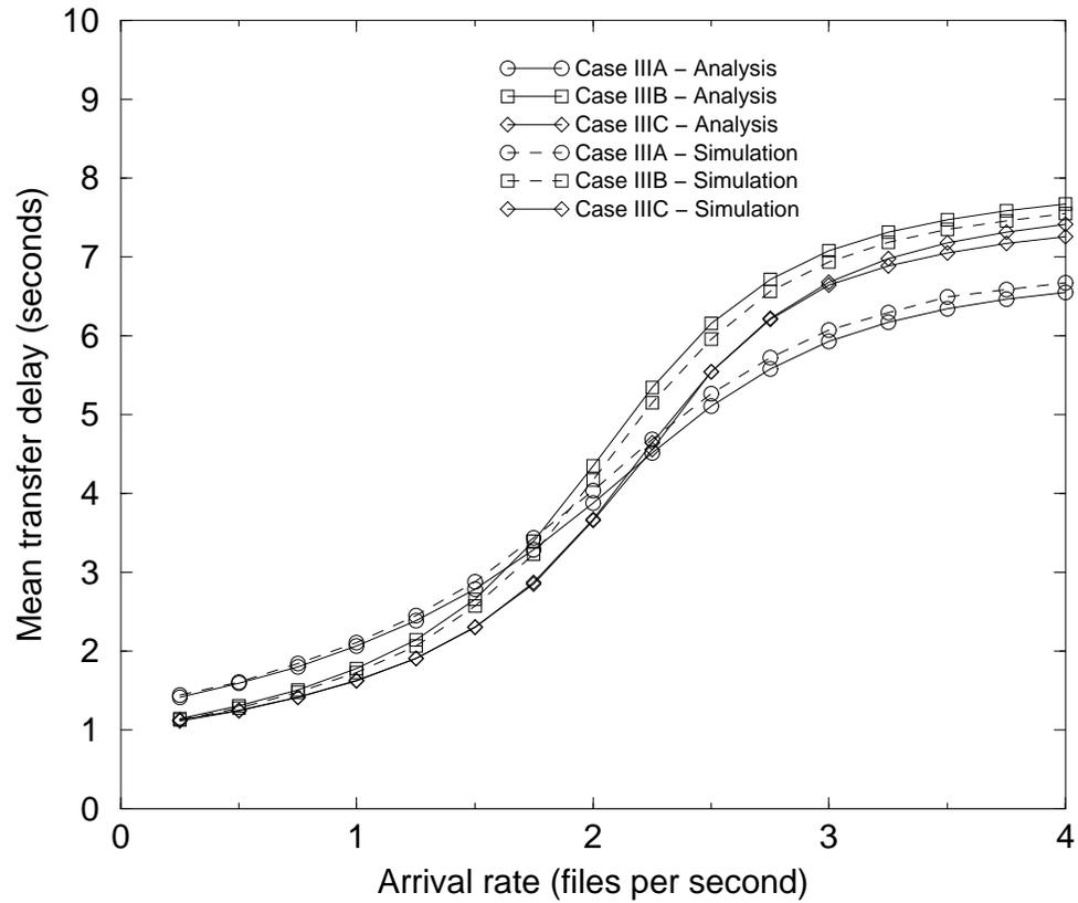
**Mean transfer delay as function of file arrival rate for Cases IIIA-C with deterministic file size**
