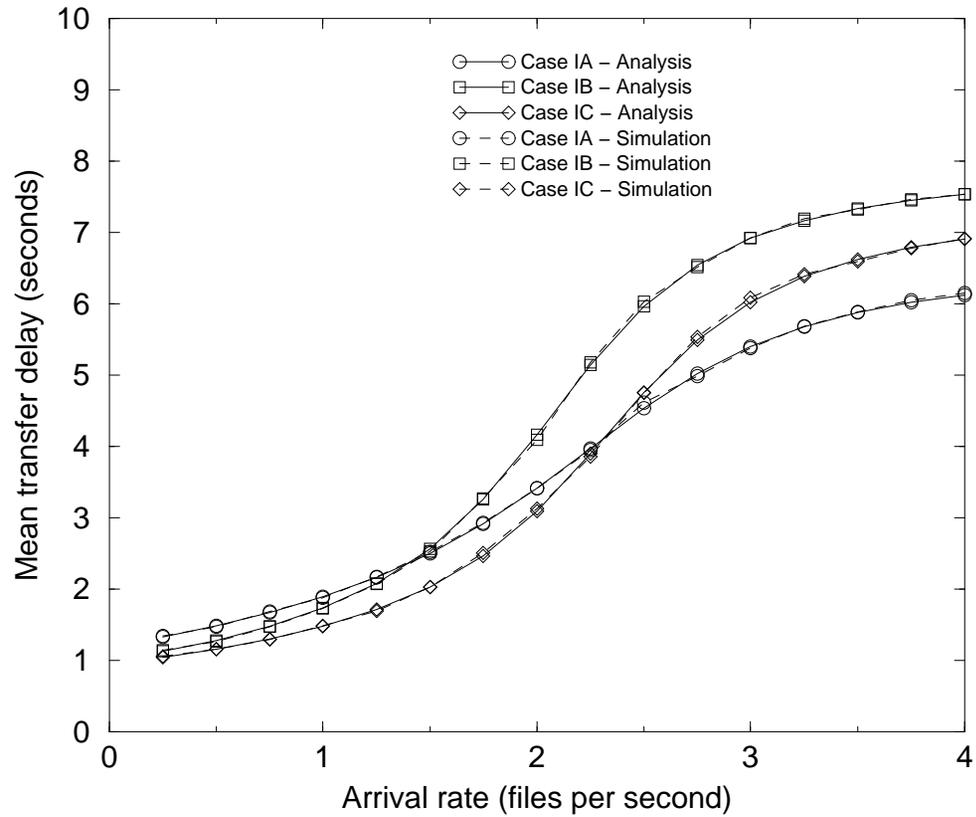
**Mean transfer delay as function of file arrival rate for Cases IA-C**
