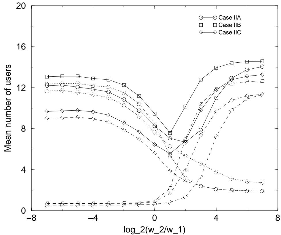
**Mean total number of users (solid line), class-1 users (dashed line), and class-2 users (dotted line) as function of  $\log_2(w_2/w_1)$  for cases IIA-C**
