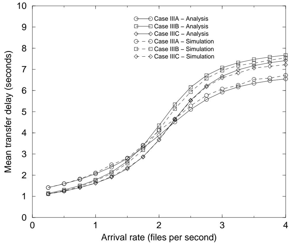
**Mean transfer delay as function of file arrival rate for Cases IIIA-C with exponentially distributed file sizes**
