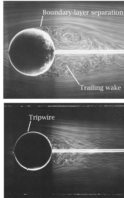
**Figure 4** Flow past a smooth sphere, clearly exhibiting boundary-layer separation and the resulting trailing wake. A tripwire has been added to the lower sphere. The resulting turbulence in the boundary layer delays separation and so leads to a smaller trailing wake. (Photos from *An Album of Fluid Motion*, Milton Van Dyke.)
